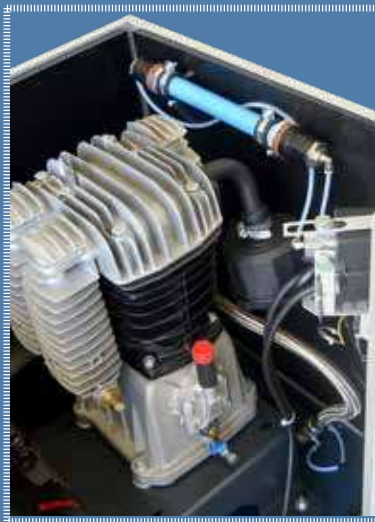
Pressure Control Tube Direct connection to air circuit.
